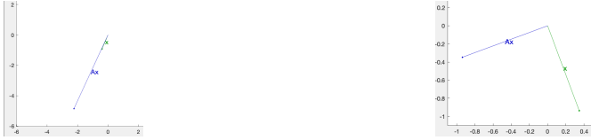
Figure 1: The left image demonstrates \mathbf{x} (green vector) as an eigenvector of matrix \mathbf{A} , transforming into \mathbf{Ax} (blue vector) as a scaled version of \mathbf{x} . The right image shows that the green vector is not an eigenvector of \mathbf{A} , as its transformation \mathbf{Ax} (blue vector) does not maintain the same direction as \mathbf{x} .
